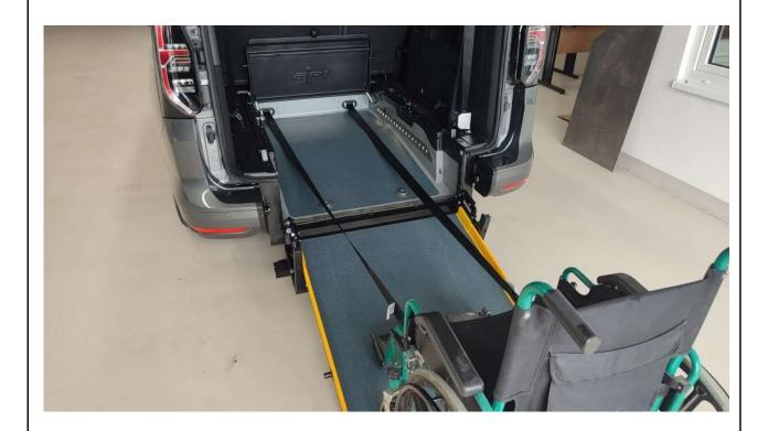
Pull out the front Retractors and make sure they are straight. Hook it on the wheelchair. No guarantee can be given for damage resulting from non-observance.
