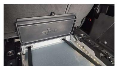
Lock the cover plate to the rear seat turning the lock to the left or right by 180°
