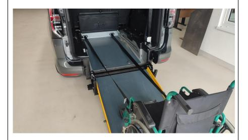
Pull out the front Retractors and make sure they are straight. Hook it on the wheelchair.
