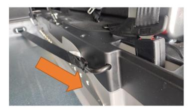
Select a fixing point at which the wheelchair can also be secured in the vehicle. Also refer to the manual of the wheelchair for specified anchoring points.
