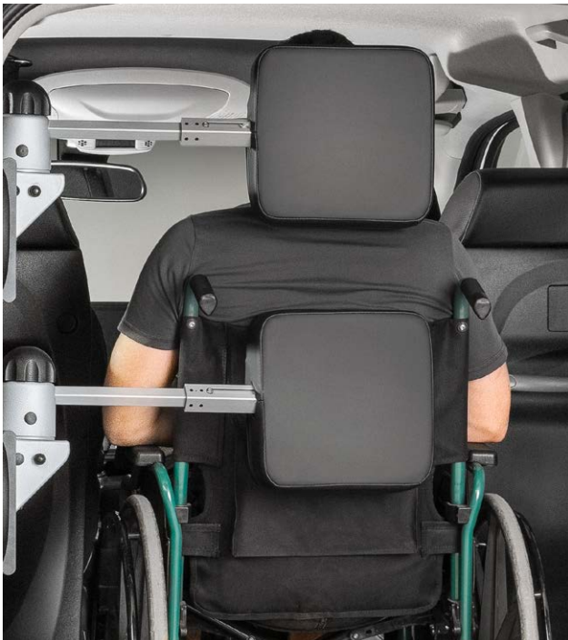
The unique patented rear impact protection system significantly increases the safety of the vehicle occupants.
