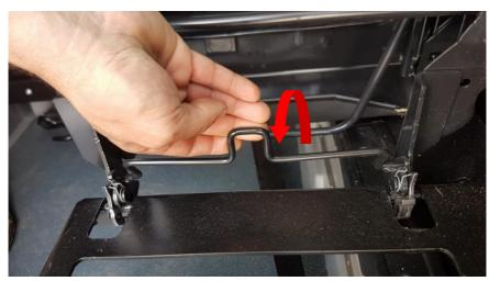
Remove the seat, push the seat console down, pull the safety pin out of the folding console and fold it 90° upwards. Ind the upper position the safety pin locks the console automatically. Make sure you hear a "click".
