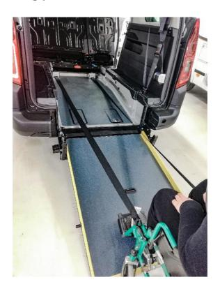
Pull out the front Retractors and make shure they are straight. Hook it on the wheelchair.
