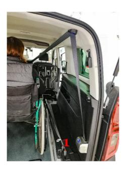
Make sure that the 3-point belt system described here is only used to secure persons seated in the loaded wheelchair. The belts must be used close to the person, must not be released while driving and all safety regulations of the vehicle manufacturer must be observed.
