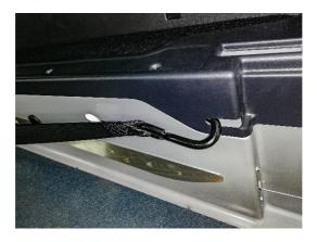
Select a fixing point at which the wheelchair can also be secured in the vehicle. Also refer to the manual of the wheelchair for specified anchoring points.
